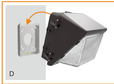
Lift the fixture up and tilt it slightly towards the wall mount bracket as figure D shown. Hook the fixture base plate to the mounting bracket.
