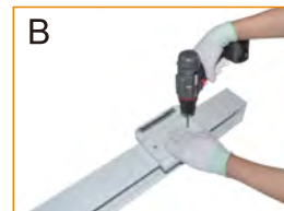
B Following the template, secure the base plate onto the fixture
